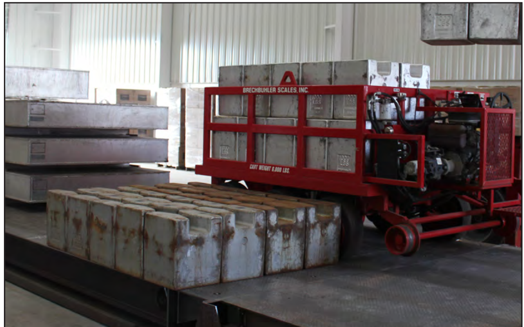
Testing with block and slab weights.
