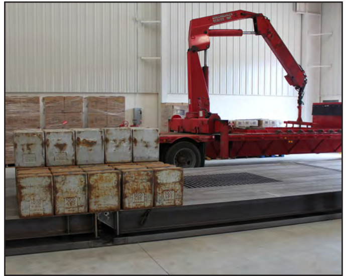
NTEP testing with smaller 1,000 lbs block weights
