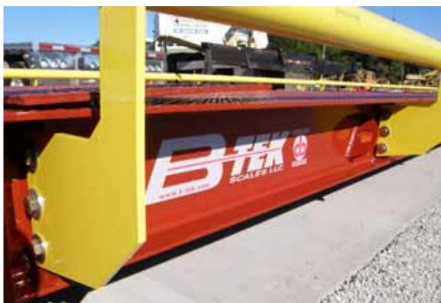
Figure 4 offers a view of the bolt-on-site sight rails. The rails are a visual guide for the truck operators to indicate the sides of the truck scale.
