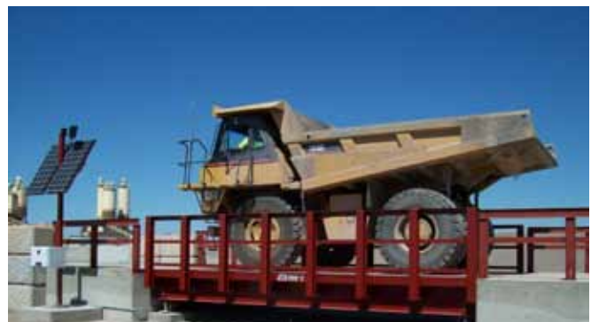
Figure 4 is the finished scale shown with the solar panel
