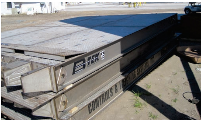
Figure 5 of new scales ready to install
